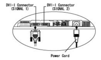
To input the Signal through ADC
